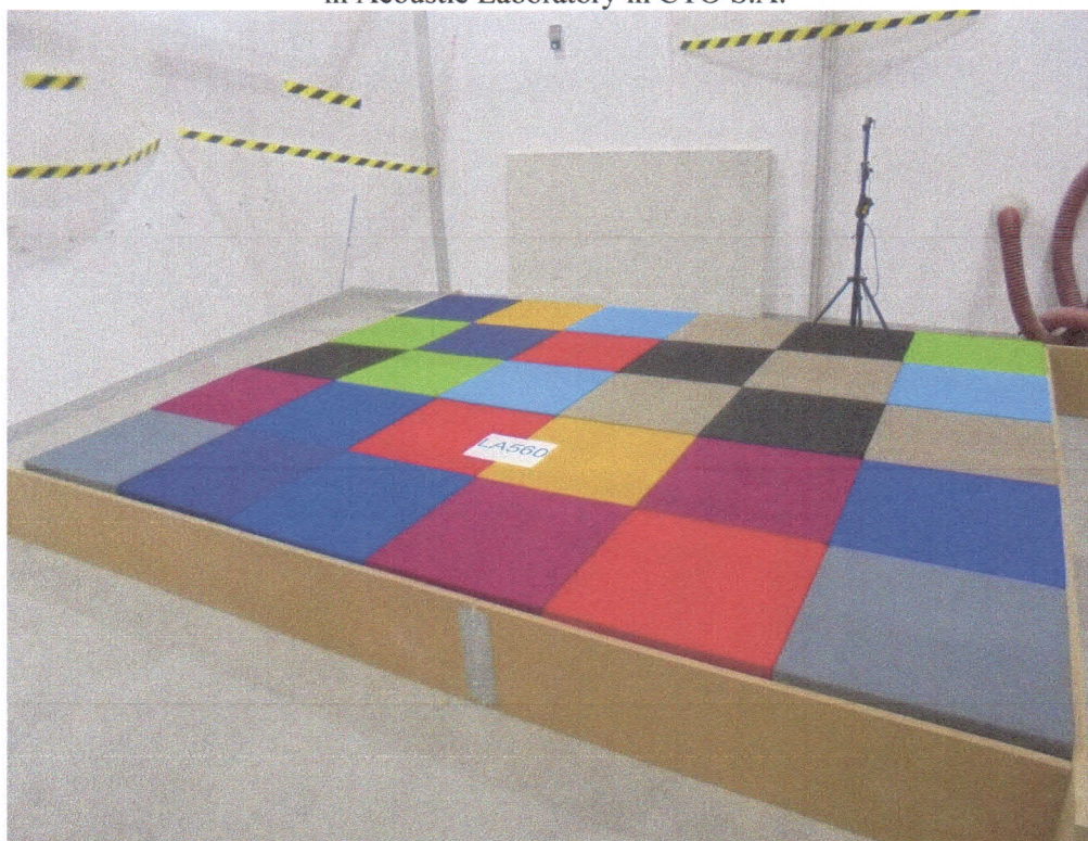
Fig. 2. Test object LA560, Creative Design Szymon Rychlik acoustic panels, in reverberation chamber in Acoustic Laboratory in CTO S.A.
