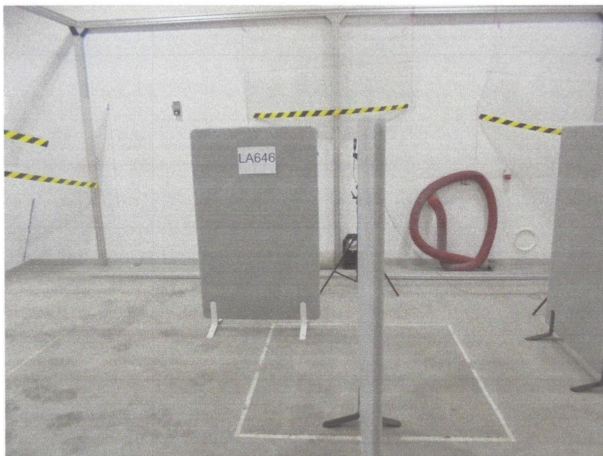
Fig. 2. Test object LA646 photo, "Creative Design Group Szymon Rychlik" acoustic panels, in reverberation chamber in Vibroacoustic Tests Laboratory in CTO S.A.
