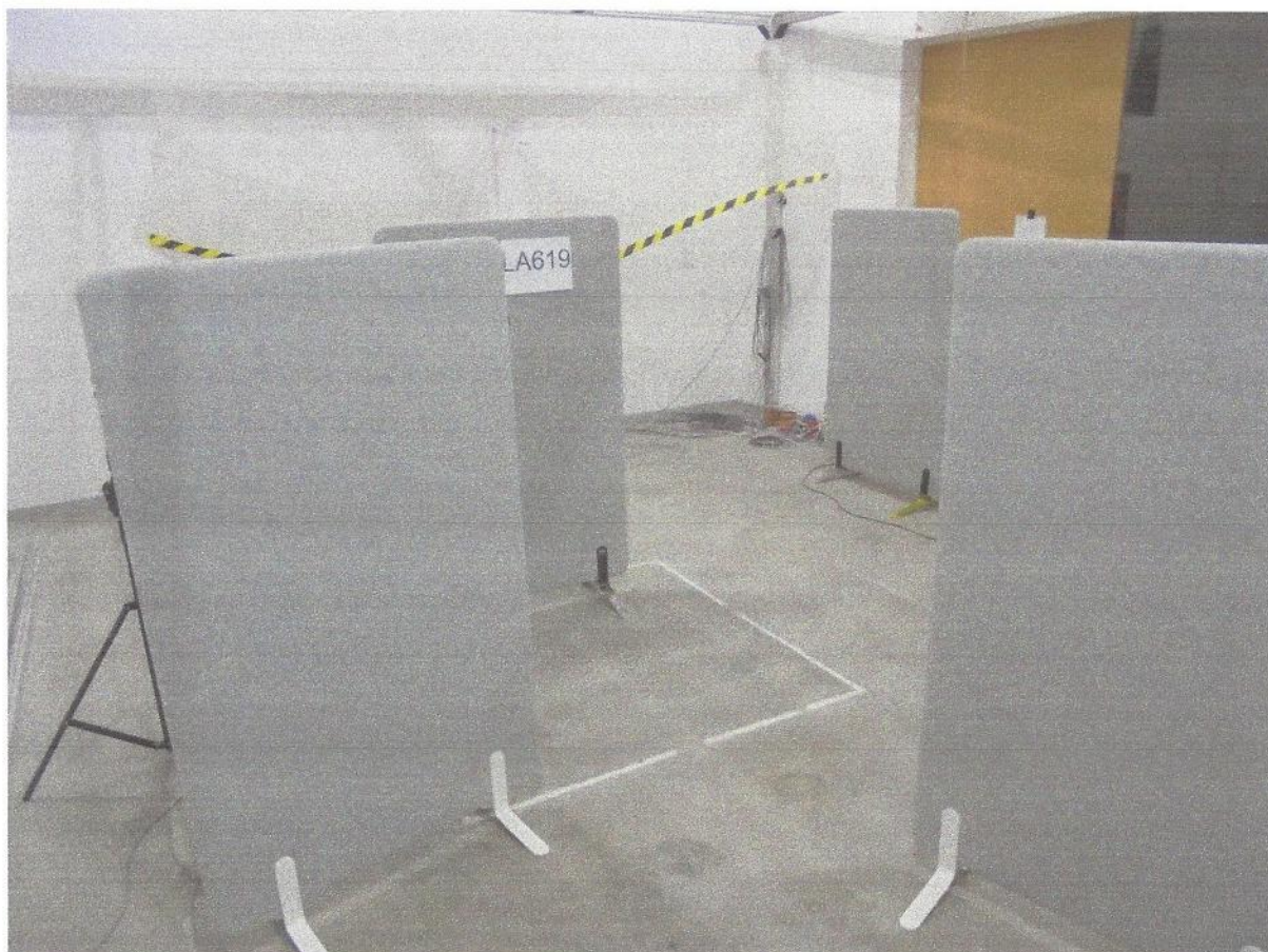
Fig. 1. Test object LA619 photo, "Creative Design Group Szymon Rychlik" acoustic panels, in reverberation chamber in Vibroacoustic Tests Laboratory in CTO S.A.
