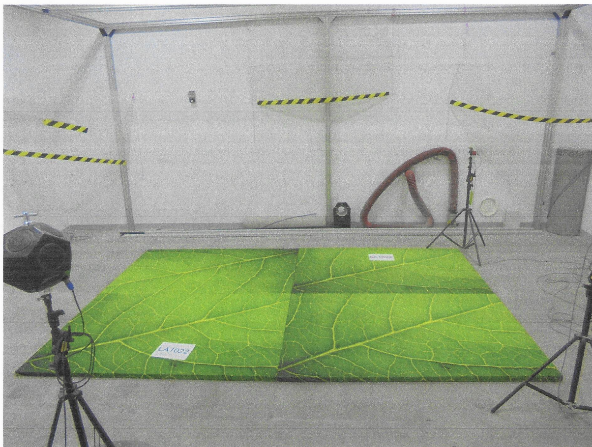
Fig. 1. Test object LA1022, absorbing panels with print PRINT by HUSH CREATIVE DESIGN GROUP in reverberation chamber in Acoustic Laboratory in CTO S.A.
