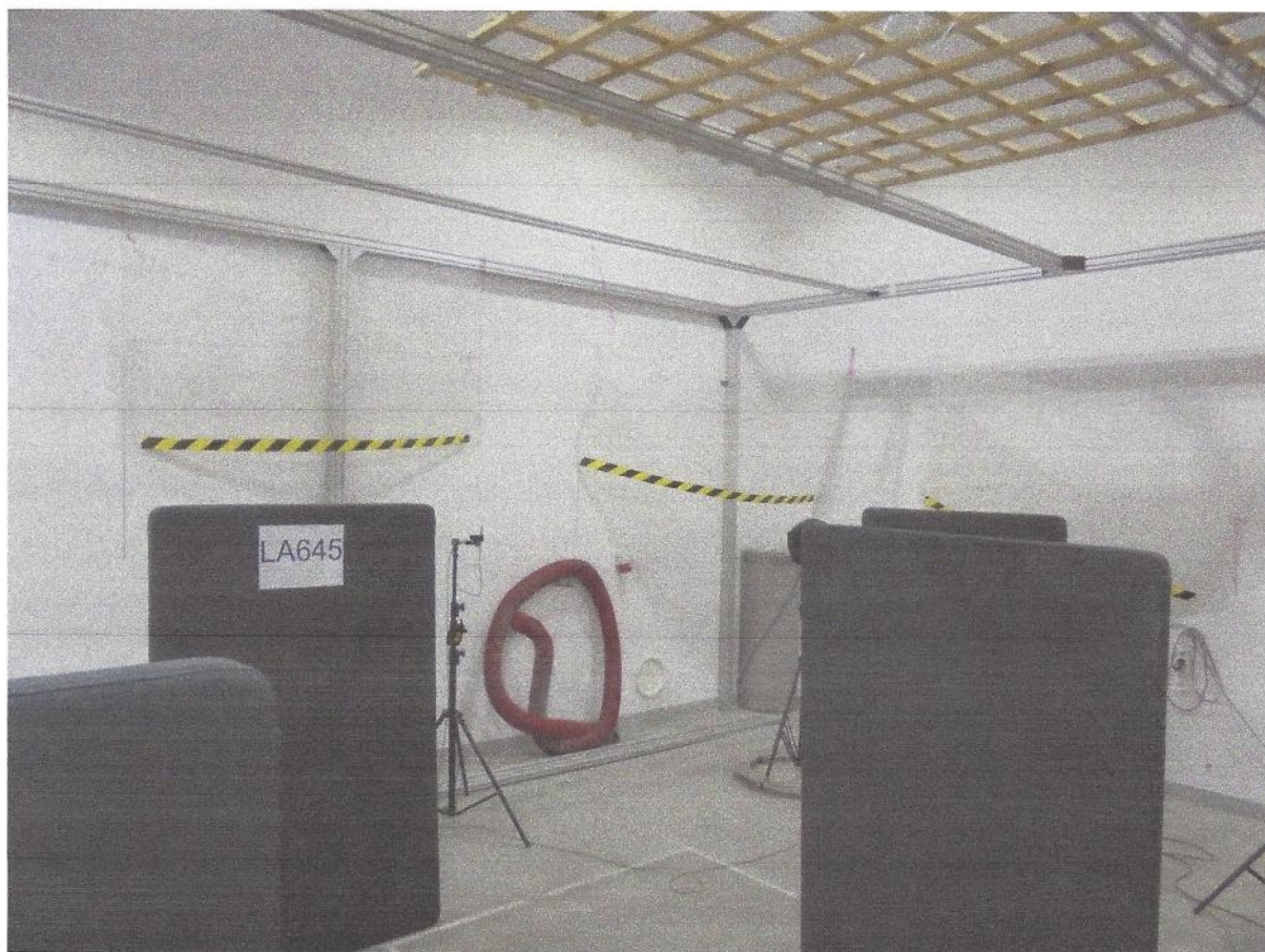
Fig. 1. Test object LA645 photo, "Creative Design Group Szymon Rychlik" acoustic panels, in reverberation chamber in Vibroacoustic Tests Laboratory in CTO S.A.
